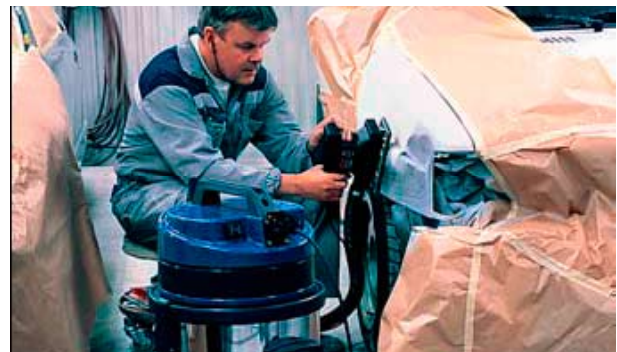
A mobile high vacuum unit with a sander or grinder can be a flexible alternative for smaller jobs.
